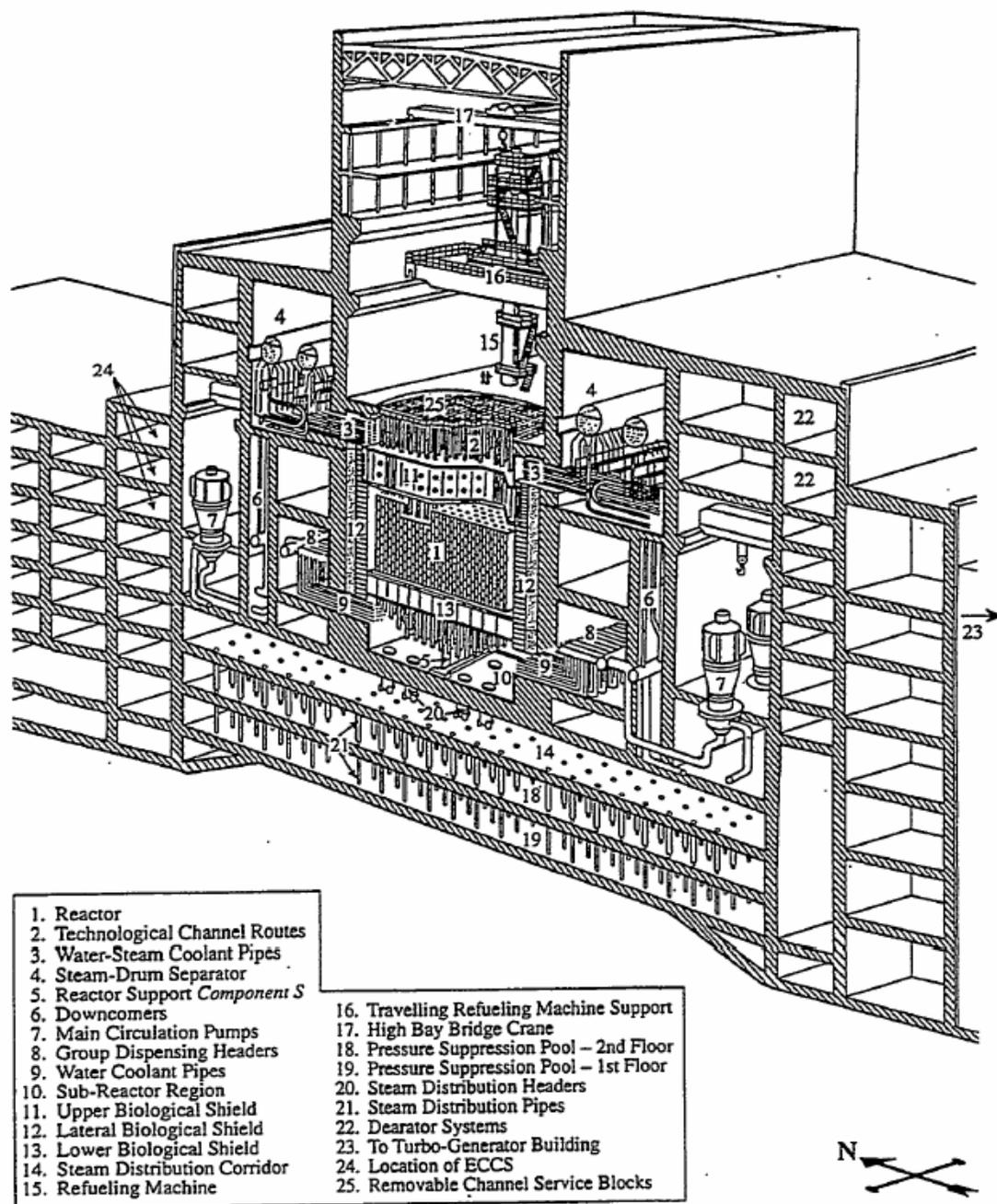
Figure 1: Intact Chernobyl Unit 4 Cross-Section<sup>6</sup>
