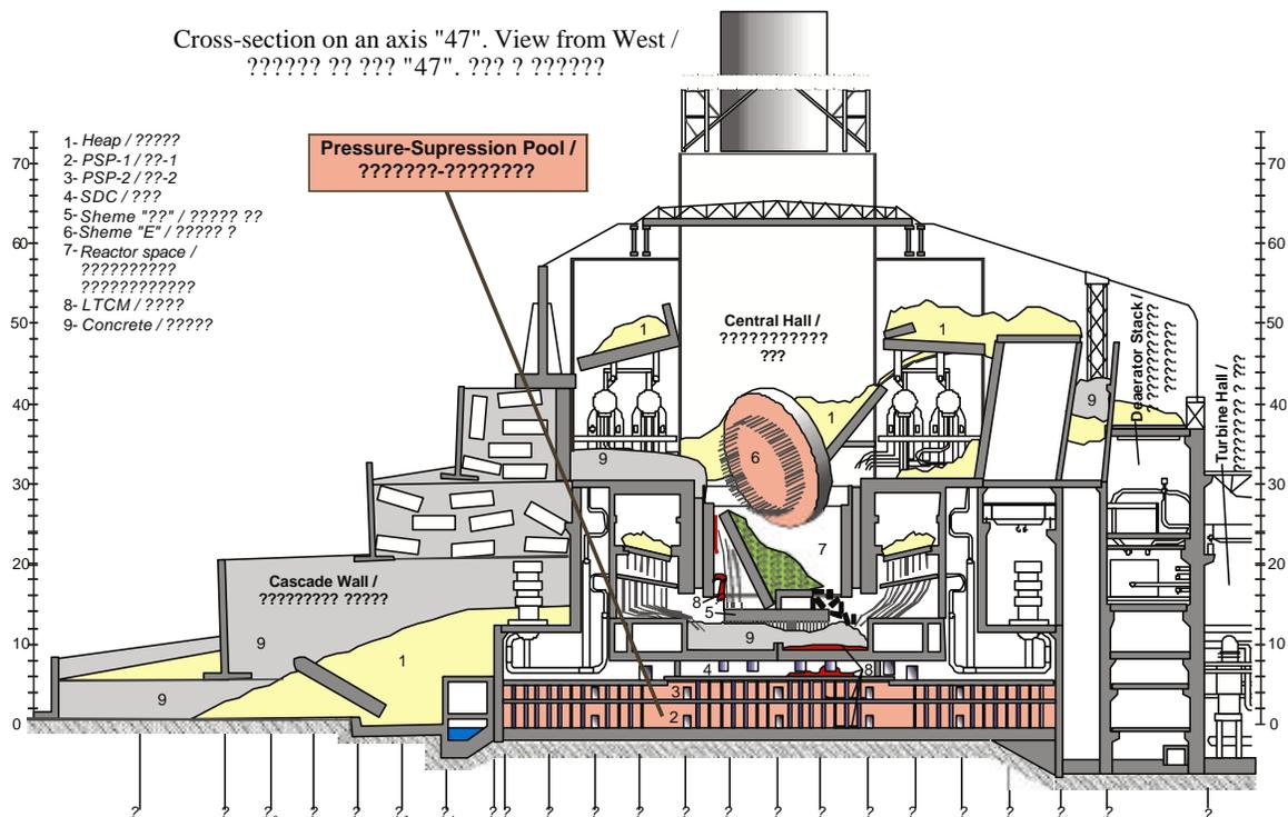
Figure 3: Chernobyl Unit 4 Shelter Cross-Section<sup>1</sup>
